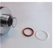
Unscrew the knurled nut from each end of the chamber. Remove the PTFE slip ring and O ring from both ends of the chamber.
