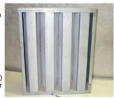
All **DISCARB** products may be supplied with a single face seal on request. As the product is omni-directional in terms of airflow, this suffices as either a clean or dirty air side gasket. If required two gaskets can be fitted. **Discarb** units may be supplied as standard capacity units with 20mm panels or heavy Duty in which case 25mm thick carbon panels will be fitted.
