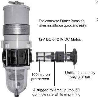
All Racor filter materials and seals are compatible with ultra-low sulphur diesel (ULSD) fuel and B2 to B20 Biodiesel. See Racor bulletin 7679.
