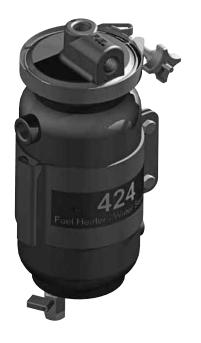
Want proven reliability? A Racor 424 Fuel Heater/Water Separators are for today's high performance heavyduty and smaller midrange engines. These lightweight aluminum units use engine coolant to produce a 47° F rise in fuel temperature, eliminating the need for fuel blending.
